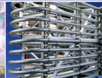
HIGH PRESSURE PRODUCT COOLER Pre-assembled unit PN 230 MPa
