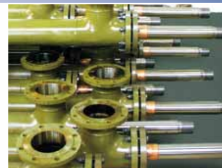
INTERSTAGE COOLER High pressure jacketed tubes with copper-cladding, PN 160 MPa
