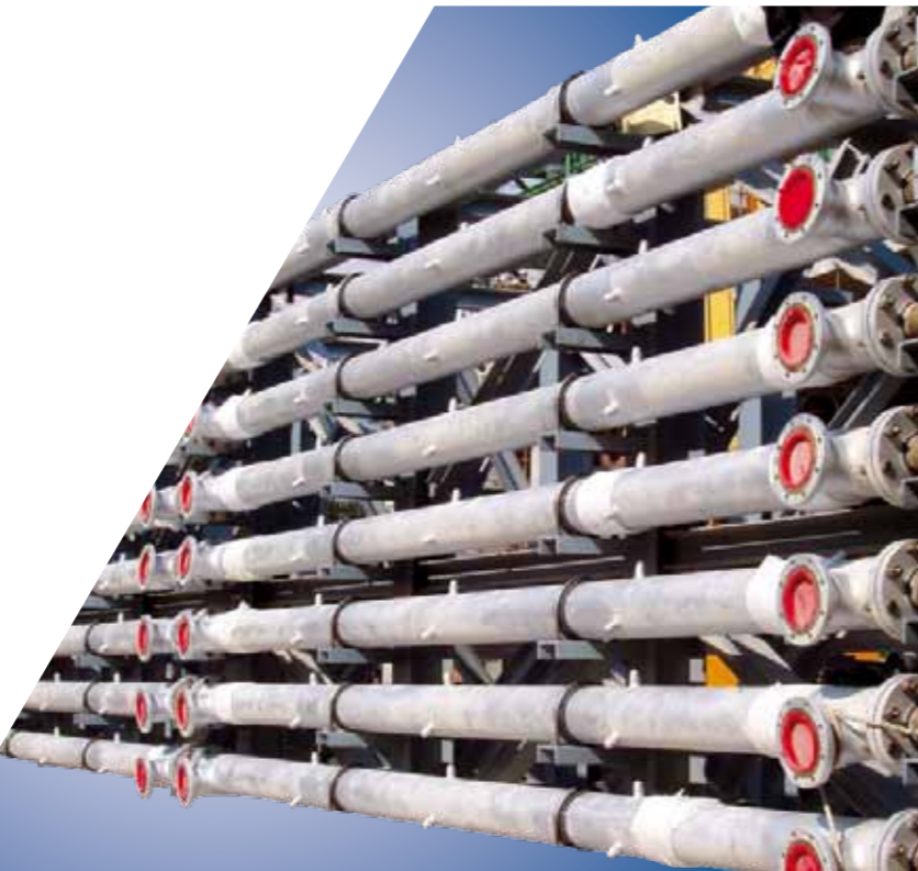
HYPER COMPRESSOR INTERSTAGE COOLER (under construction) PN 160 MPa
