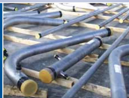
PREFABRICATED ISOMETRICS up to NS 10" 25Cr-22Ni-2Mo (Böhler A405)
