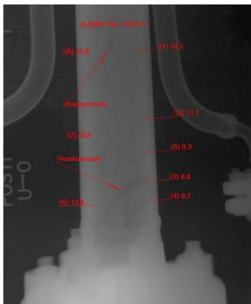
Picture 8: Digital Radiography film of the 3" pipe line
