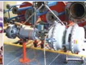
VALVE TEST FACILITY: BHDT has its own control valve testing facility. NP0.6 MPa to 250 MPa, NS up to 300 mm • Flow coefficient KV (Cv), characteristics • Media pressure drop factor FI • Leak test Pressure upstream of the valve • Pressure downstream of the valve • Pressure drop • Stroke position • Flow rates 0,5 up to 1300 m 3 /h (0,13 up to 340 gal/h)
