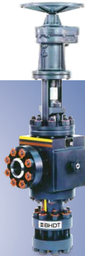
ANGLE VALVE stub ends, steam jacket NS 5", PN 18.5 MPa SA182 F316LUG (Böhler A220)
