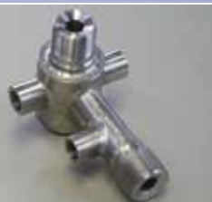
VALVE BODY FOR ANGLE VALVE NS 1", PN 25 MPa Duplex
