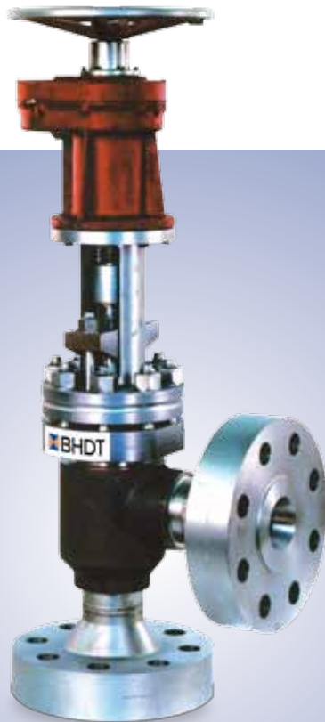
ANGLE VALVE gear operated, NS 6", weld neck flange, PN 2500 lbs SA182 F316LUG (Böhler A220)
