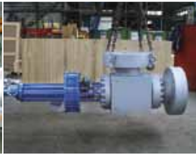
CONTROL VALVE NS 16", PN 25 MPa SA182 F316LUG (Böhler A220)
