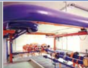
VALVE TEST FACILITY: BHDT has its own control valve testing facility. NP0.6 MPa to 250 MPa, NS up to 300 mm • Flow coefficient KV (Cv), characteristics • Media pressure drop factor FI • Leak test Pressure upstream of the valve • Pressure downstream of the valve • Pressure drop • Stroke position • Flow rates 0,5 up to 1300 m 3 /h (0,13 up to 340 gal/h)
